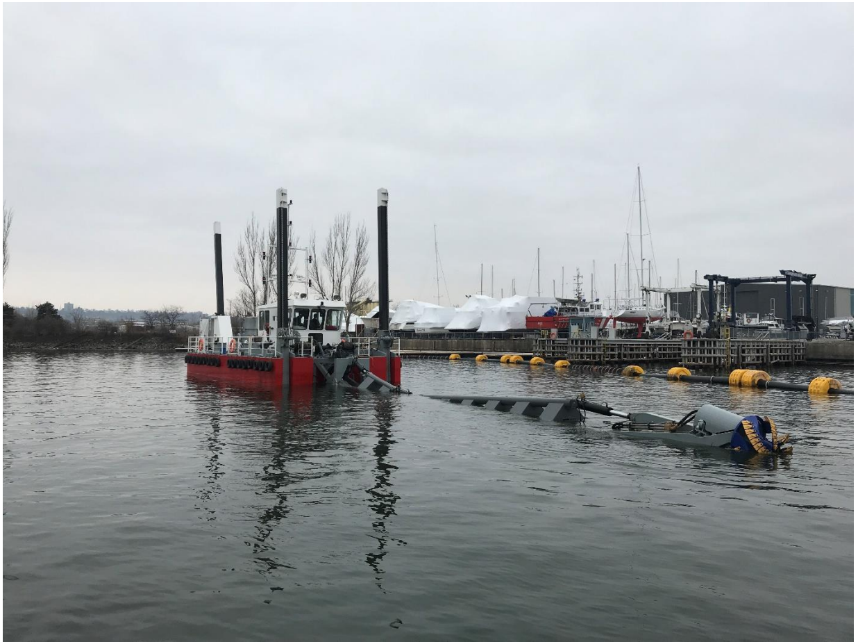
14" Self-Manoeuvring Cutter Suction Dredger, typisch product from De Hollandsche IJssel
